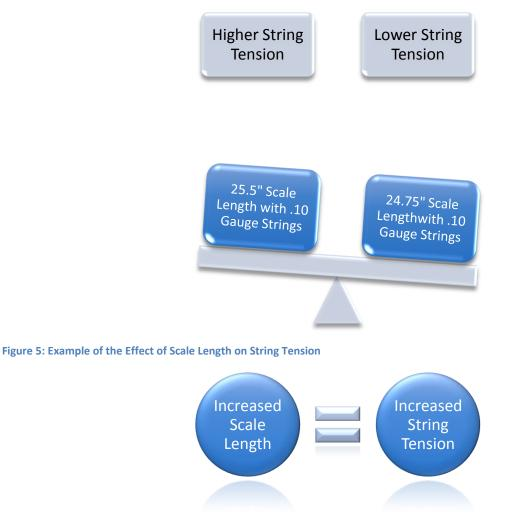
Figure 6: Relationship between Scale Length and String Tension when String Guage and Pitch is kept Constant
