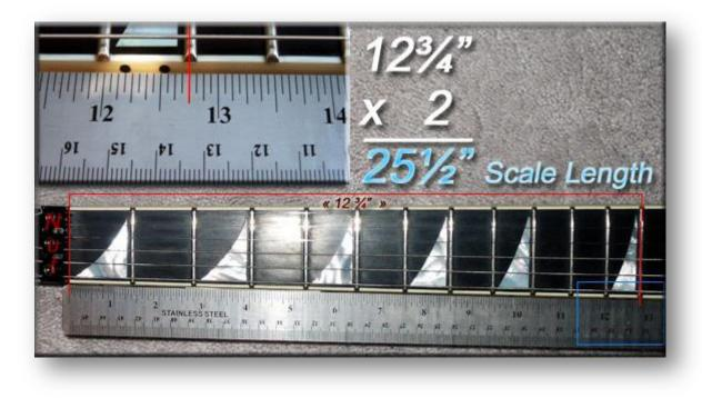
Figure 2: Measuring the Scale Length of Jackson Soloist Note: When taking this measurement, the ruler should be perpendicular to the frets and nut. In this illustration, the ruler has been placed parallel to the edge of the neck for clarity.
